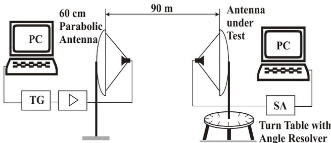
Fig. 3. Experimental setup for radiation pattern measurement.
