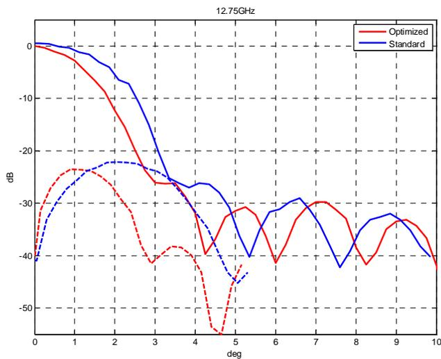
Fig. 6. Measured Antenna Radiation Patterns at 12.75GHz
