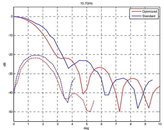
Fig. 4. Measured Antenna Radiation Patterns at 10.7GHz.
