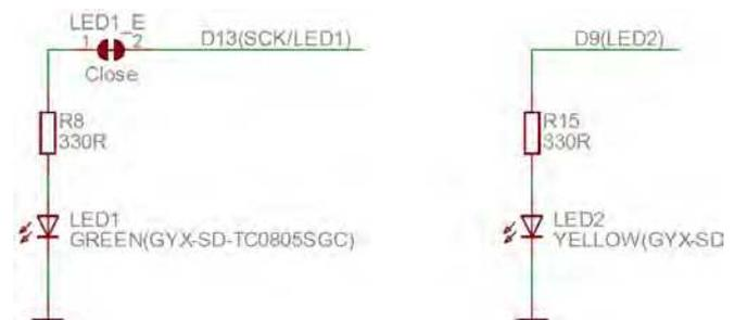
Fig.2. Light emitting diodes connected to ATmega328P pins 17 (LED1 - digital signal D13) and 13 (LED2 - digital signal D9).
