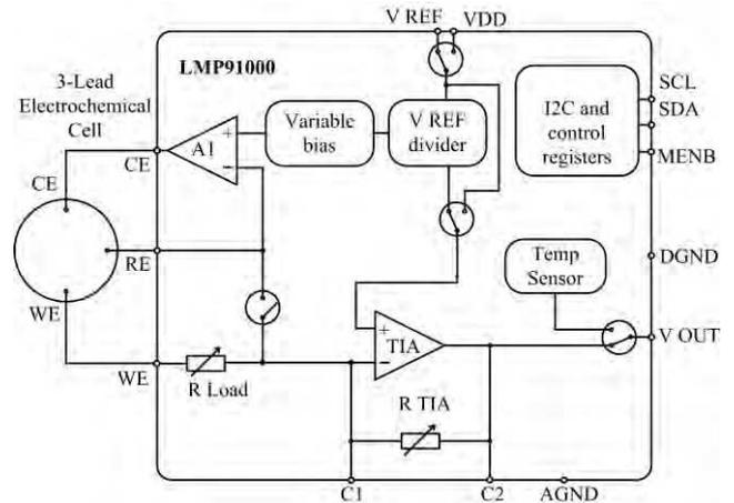
Fig. 2. Functional block diagram of LMP91000.
