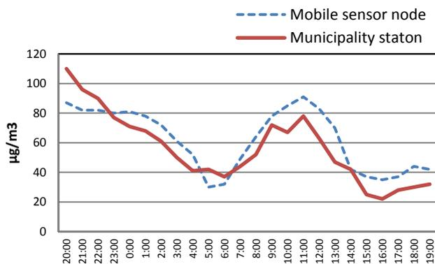
Fig. 4. Comparing the data for the daily course of NO<sub>2</sub> concentration measurement (averaging each hour): values provided by the municipality station and a mobile sensor node.
