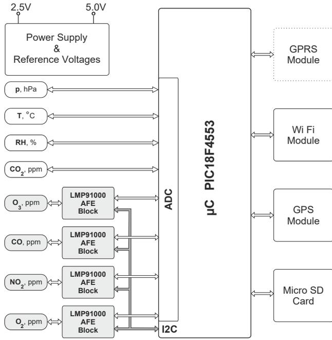
Fig. 1. Block-diagram of the developed node.
