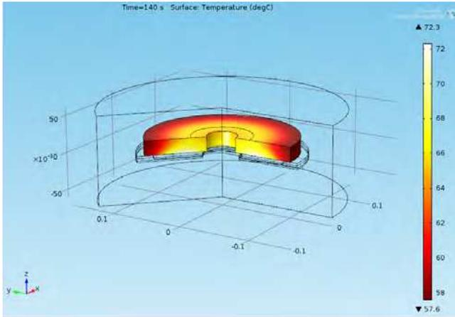
Fig. 3. Distribution of the temperature field in the detail.
