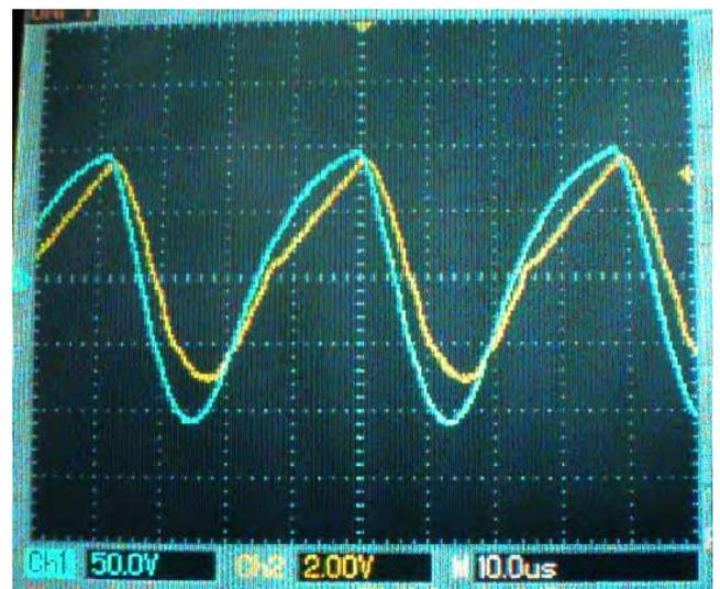
Fig. 8. Inductor voltage (blue) and current through the coil (yellow).
