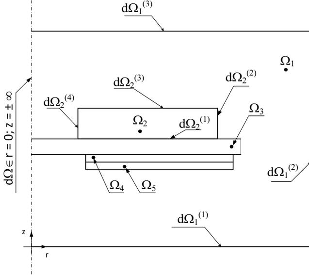
Fig. 1. The geometry of the model.  $\Omega_1$  – the air,  $\Omega_2$  – the detail;  $\Omega_3$  – the pyro ceramic plot;  $\Omega_4$  – the inductor;  $\Omega_5$  – the magnetic concentrator.
