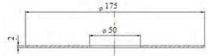
Fig. 6. The Dimensions of the inductor
