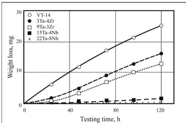
Fig. 1. Relation between mass loss of materials in the boiling solution of nitric acid and duration of testing.
