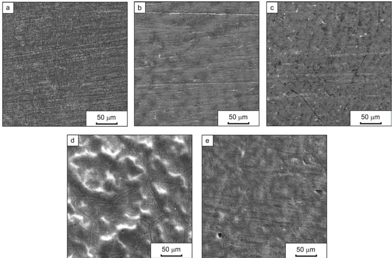
Fig. 2. Surfaces of the samples after corrosion tests in the boiling concentrated solution of nitric acid: a – VT14 titanium alloy; b - 15Ta-4Nb alloy; c –22Ta-8Nb alloy; d –3Ta-4Zr alloy; e –9Ta-3Zr alloy.
