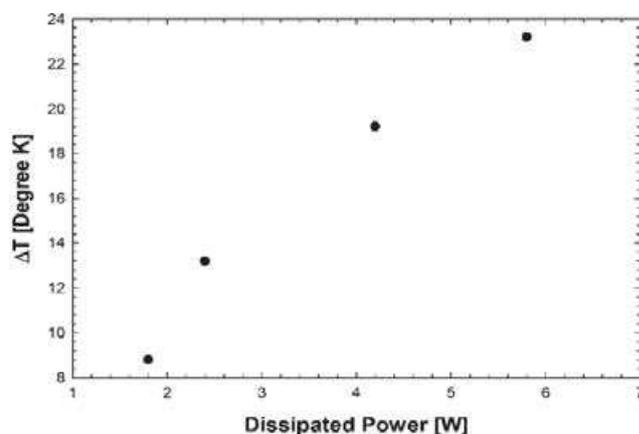
Figure 4. Increase of sample temperature versus plasma dissipated power.
