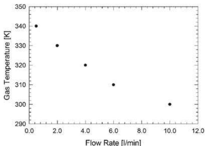
Figure 3. Gas temperature versus gas flow rate for power of 10W [7].
