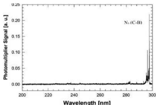
Figure 5. UV spectrum of a DBD in air in the 200-300nm wavelength range [7].
