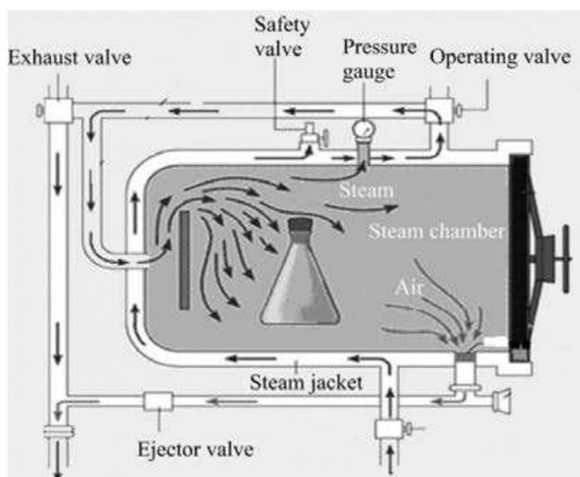
Figure 1. An Autoclave.
