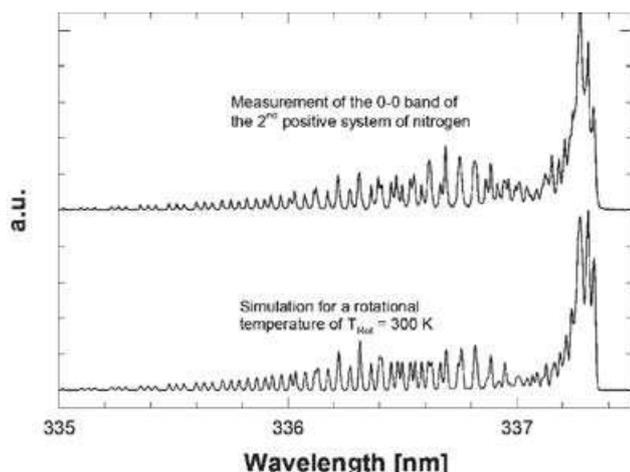
Figure 2. Measured and calculated rotational bands of 0–0 transition of the second positive system of nitrogen. The spectra are intentionally shifted vertically for better comparison [7].
