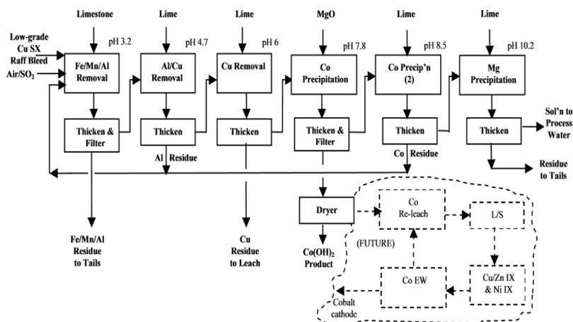
Fig. 4. A typical flowsheet of a cobalt section (Fisher, 2011).
