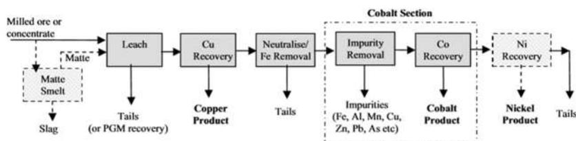
Fig. 3. Generic Cu/Co/Ni recovery flowsheet (Fisher, 2011).
